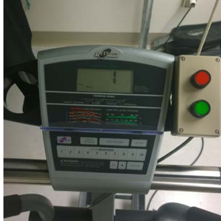
Figure 2-5: Red emergency button on the right side of the elliptical that the subject can press in case there is a need to stop the rotation of the footplates.
